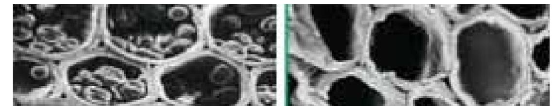
Bamboo on molecular level before (left) and after(right) the density-thermo treatment: before the sugar molecules are still visible, after the treatment they have disappeared. With this treatment bamboo is no longer a feeding place for fungi and micro-organisms.
